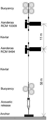
**Figure 1.** Calibration rig. Vertical distances not to scale.
