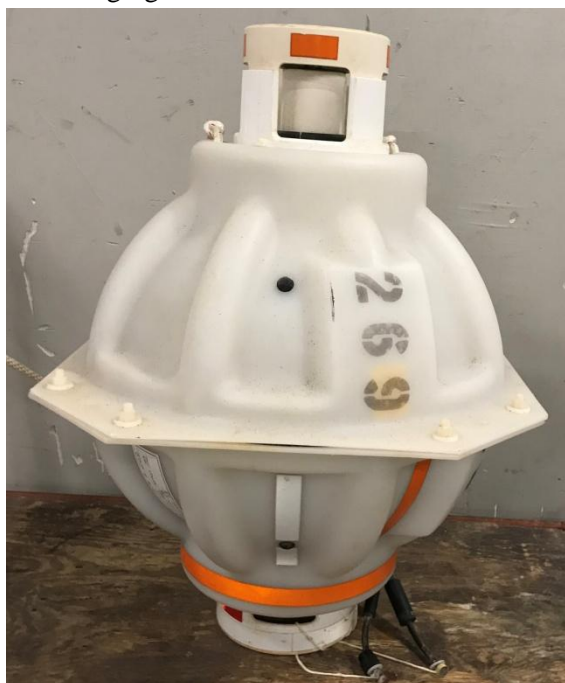
Figure 3.1. One of the PIES (P-269) that was used in the 2017-2019 experiment. The PIES is mounted on an anchor frame and deployed on the bottom. The measurements are stored in the instrument and may be uploaded to a research vessel acoustically or retrieved after the PIES has been released from the frame and recovered.
