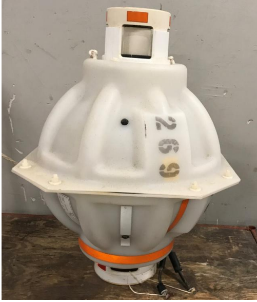
Figure 6. One of the PIES (P-269) that was used in the experiment. The PIES is mounted on an anchor frame and deployed on the bottom. The measurements are stored in the instrument and may be uploaded to a research vessel acoustically or retrieved after the PIES has been released from the frame and recovered.
