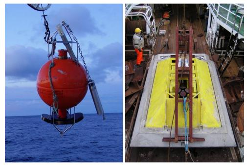
**Figure 2.2** Left photo: A 75 kHz RDI Broadband ADCP in a Flotation Technology buoy with microcat and acoustic release about to be recovered in the Faroe Bank Channel. Right photo: A 150 kHz RDI Broadband ADCP in a buoyant aluminium frame (yellow), mounted on a concrete anchor, ready to be lowered to the bottom attached to a special deployment frame (brown).
