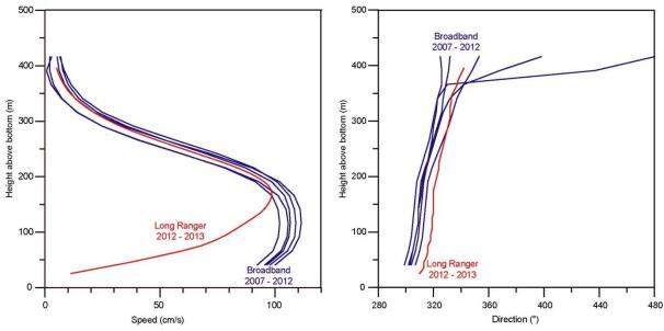
**Figure 1.** Average profiles of vectorially averaged speed (left) and direction (right) for six ADCP deployments at site NWFB from summer 2007 to summer 2013 using Broadband (blue curves) and Long Ranger (red curve) ADCPs.
