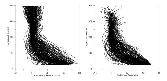
**Figure 8.** Variation of the Long Ranger error  $v_{err}(z,t)$  (left) and its relative value  $v_{err}(z,t) / v_{adj}(z,t)$  (right). Each trace represents one day in the 2012 – 2013 deployment period. Relative error is not plotted when  $v_{adj}(z,t) < 30$  cm/s.
