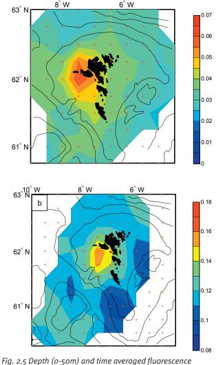
Fig. 2.5 Depth (0-50m) and time averaged fluorescence from the biological oceanography cruise in late April/early May (a, 1994-2008) and from the O-group survey in late June/early July (b, 1990-2008). The red crosses show the grid, on which the station data are gridded onto.
