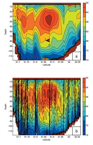
Fig. 4.6 Back-scatter data (dB) from the ship-mounted echo-sounder along the Suðuroy-Mykines section (see Fig. 4.5c). Subsampled (EchoView) at a) 10 minutes and b) 1 minute intervals (Suðuroy to the left and Mykines to the right). The vertical lines result from hydrographic stations taken along the section, when the ship is halted.
