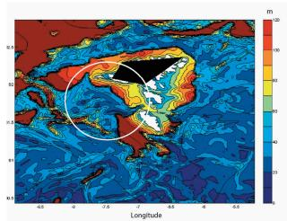
Fig. 4.36 Simulated mixed-layer depths on May 5, 2000, using HYCOM. The inflowing filaments of stratification from the Western region and onto the shelf are emphasized within the white circle.
