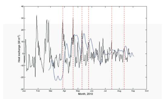
Fig. 4.17 The ADCP backscatter at FASB averaged over the deepest 10 bins (blue, low-passed), and the air-sea heat exchange from the Western region (black). Increased heat loss to the atmosphere is upward. The seasonal cycle has been removed and daily values are shown (which means that the values are relative). The linkage between positive heat loss anomalies and increased backscatter is emphasized with the red dashed lines
