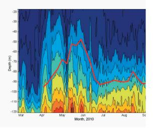
Fig. 4.16 Backscatter intensity (colors) from the bottom mounted ADCP at station FASB, and the chlorophyll concentration at coastal station 'Skopun' (red), not to scale and shifted four days forward in time.
