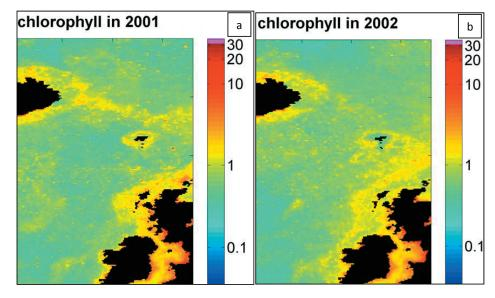
Fig. 2.4 Sharp decline/increase in phytopankton abundance in shelf/open-ocean water in the northeastern Atlantic from 2001 to 2002. Annual composites of surface chlorophyll concentrations as measured by the SeaWiFS satellite ( $\mu$ g chl-a  $^{l-1}$ , on a log scale).
