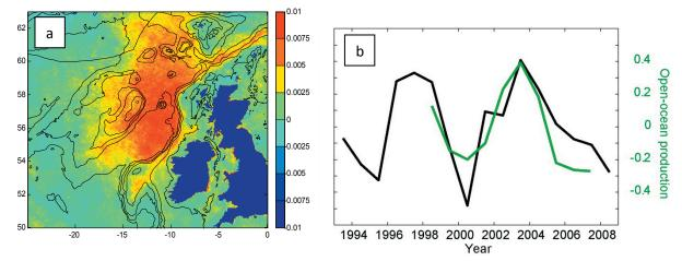
Fig. 2.2 The sub-decadal variability is evident in the surface chlorophyll concentrations. This is shown by applying EOF analysis to annually averaged chl-a data from the SeaWiFS satellite. a) The spatial pattern is shown in and b) the time series (green), plotted against the inverted and de-trended gyre index (black).
