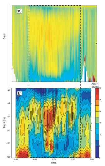
*Fig. 4.15 Back-scatter during April 24, 2010. a) output from the ship mounted echo-sounder and b) back-scatter anomaly from the bottom-mounted ADCP, with the time-average profile (Fig. 4.14b) subtracted. The dashed rectangles show the same time window. The depth in a) is approximate.*
