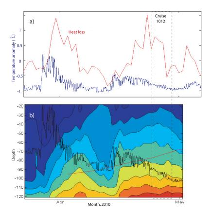
Fig. 4.18 Insight from the bottom temperature at FASB. a) The bottom temperature (blue) and the heat loss anomaly to the atmosphere (red, positive out of the ocean) and b) the backscatter intensity (as in Fig. 4.16), and the bottom temperature (black line) as in a). The dashed rectangle shows the duration of the extended leg of cruise 1012.
