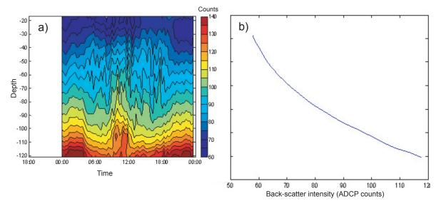
*Fig. 4.14 Back-scatter intensity from the bottom mounted ADCP at mooring FASB. a) A time-depth (Hovmöller diagram) of the intensity during April 24 and b) the time-averaged intensity for the full duration of the deployment (20 January-4 September, 2010).*
