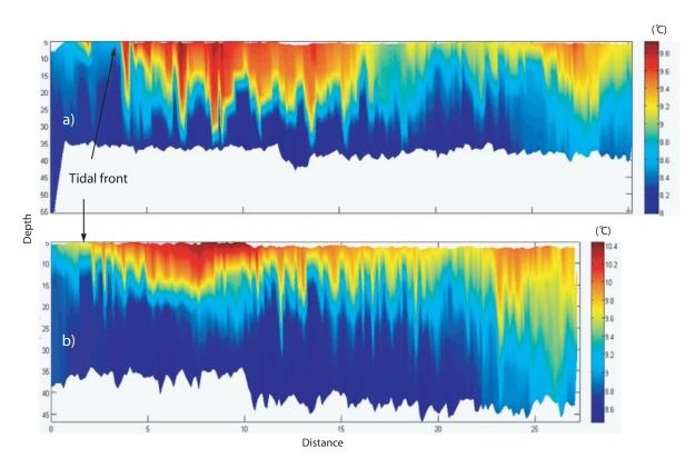
*Fig. 4.23 Two temperature sections taken along the main section MYK (see Fig. 1.1b), using the TTW, during a) June 6, 2010 and b) June 23, 2010. Mykines is to the left, and the approximate location of the tidal front is indicated.*
