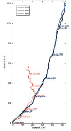
Fig. 4.21 Progressive Vector Diagram (PVD) of the nearsurface currents, sampeled by an ADCP deployed to the northwest of Suðuroy (FASC, see Fig. 1.1).
