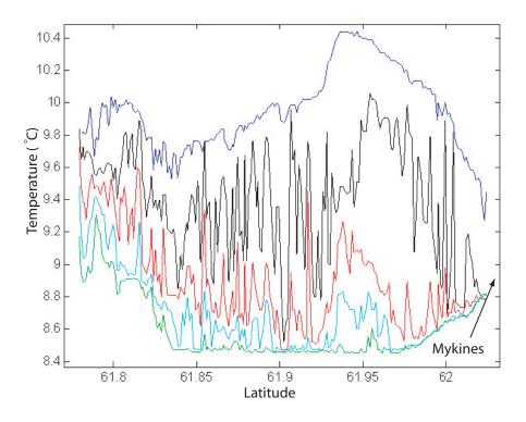
*Fig. 4.24 The temperature records from each individual temperature sensors on the TTW, located at roughly 5 m (blue), 14 m (black), 23 m (red), 32 m (light blue) and 40 meters depth (green) are plotted.*
