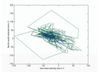
Fig. 4.20 Scatter plot of the depth averaged current velocities (all bins) at mooring FASB. The time-average (over all the full duration of the mooring) is shown with the red dot.
