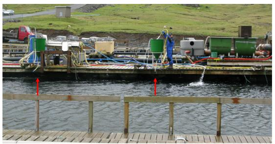
Fig. 2.2. Visualisation of the experimental setup in the eastern basin. The tank on the left hand side contained silicate while the tank on the right hand side contained the NPK fertilisers. Further to the right, inflowing seawater is discharged into the basin.
