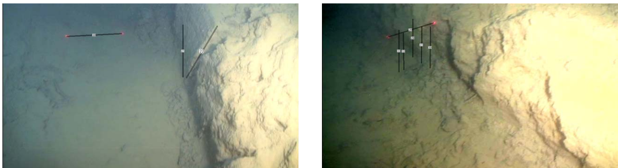
Figure 23. Tracks of door from the rockhopper trawl. The black bars shows measurements done to size the track. The distance between the red laser lights was 10 cm.
