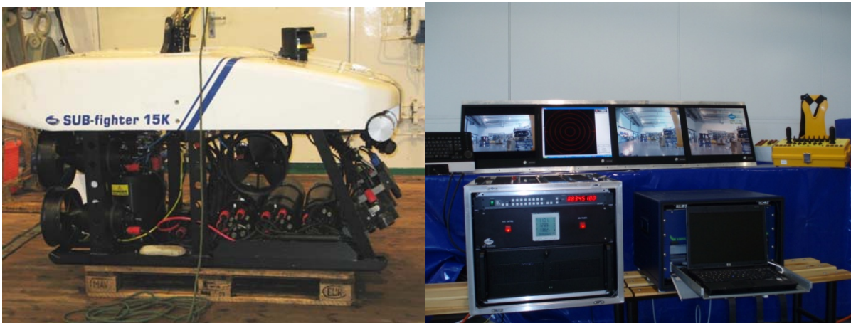
Figure 13. The ROV Subfighter 15K (left) used for bottom habitat mapping. The right picture shows the surface control equipment and observation screens.
