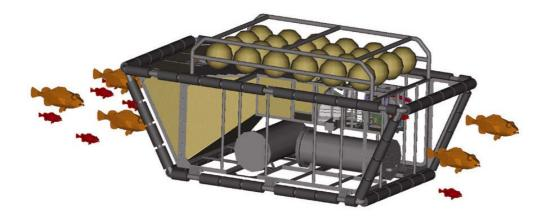
Figure 4. The newly developed Underwater Tagging Equipment (UTE) for tagging of fish *in situ*, by Star-Oddi (http://www.star-oddi.com, Iceland).
