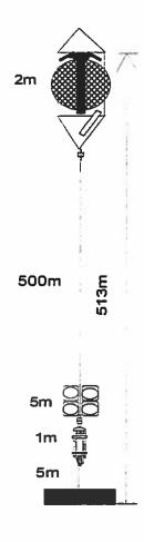
Deployment: FGEC9902 updated 1999/10/07 Instrument no.: 1644 Instrument freq.: 75 Latitude: 61 32.540 N Longitude:03 59.830 W Bottom depth: 1195 Instrument depth: 682 Center depth of first bin: 646 Bin length: 25 Number of bins: 21 Number of first ensemble: 622 Time of first ensemble: 1999 02 22 00 30 Number of last ensemble: 16378 Time of last ensemble: 1999 06 11 10 30 Time between ensembles (min.): 10 All directions have been corrected by adding: -11.0
