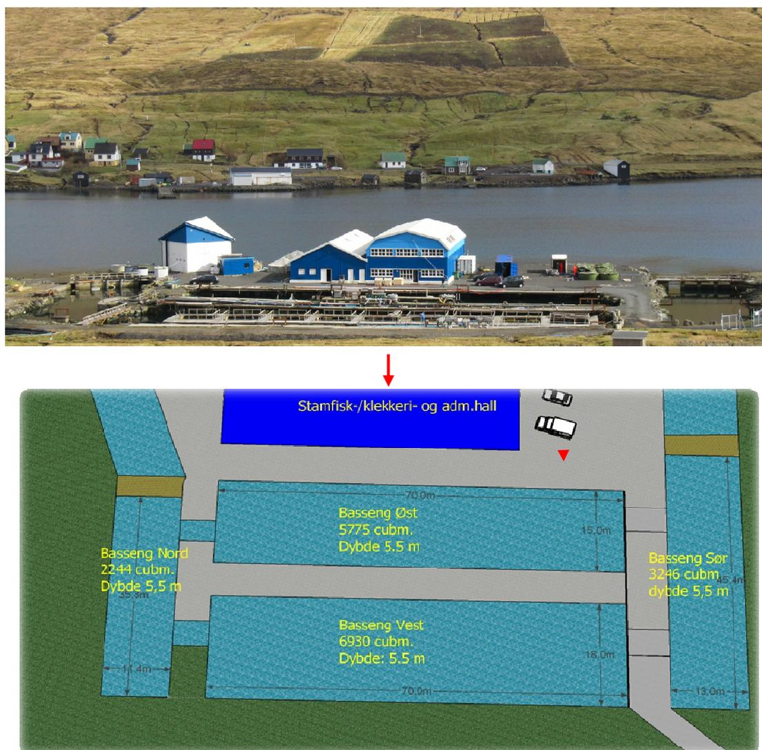
Fig. 2.1. Layout of the four basins at The Marine Station in Nesvík.
